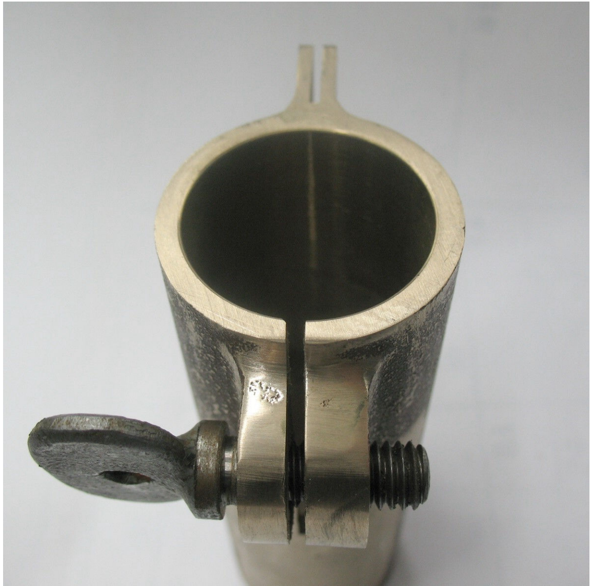
Figure 6 – Clamp collar casting with both slots cut, thumbscrew holes drilled (only one side is tapped) and thumbscrew inserted. The rib with the slot in it (shown in 12 o'clock position in photo) is for the rudder blade or fin
