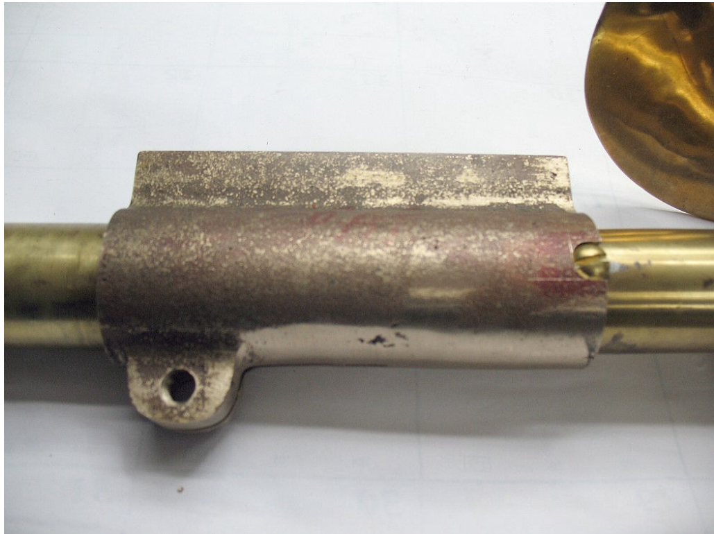
Figure 7 – Rudder yoke placed on drive shaft tube. Note the fit of the screw relief s over the head(s) of the lower unit retaining screws
