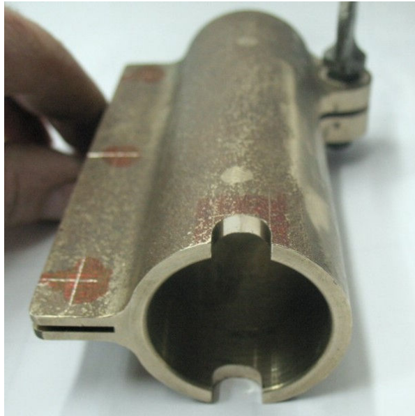
Figure 5 – Bored out casting with screw relief slots milled in and side slots already cut
